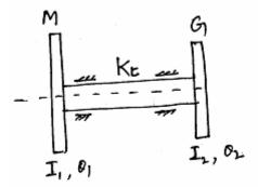
Electrical Motor – generator set is shown in the figure. Determine the natural frequencies and amplitude ratios of principal modes. [16]
